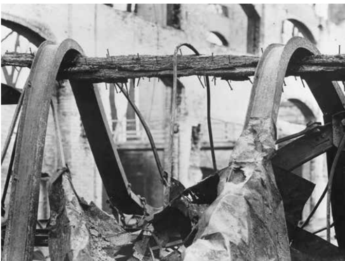
In 1953, a fire in a casein glue factory demonstrated the superior fire-endurance of untreated wood over steel.
