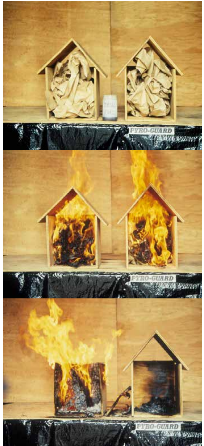
The identical contents within an untreated wood structure (left) and a Pyro-Guard® wood structure (right) were set on fire. After 15 minutes, the untreated structure became fuel and continued to burn. The Pyro-Guard® structure self-extinguished after the combustible contents were consumed, demonstrating FRTW doesn't add fuel to the fire and complies with EKOC 3.14.
