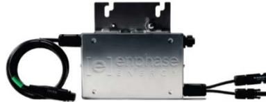
**Micro Inverters** convert dc power into ac power matching the utility voltage and frequency to generate utility quality power. They are attached to the back of a solar module. The dc circuit is the distance from the output of the solar module to the inverter, usually less than 12 inches. Disconnecting the ac utility source de-energizes most of the circuitry in a system. AC modules are in essence a National Testing Lab certified assembly of a solar module and an inverter.
