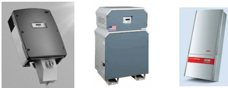
**Non Battery Inverters** convert dc power into ac power matching the utility voltage and frequency to generate utility quality power. Disconnecting the ac utility power source turns off the inverter, but DOES NOT disable the dc solar module circuit.
